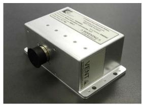
33.6Vdc, 3.3 Ah LiPo Battery Unit
